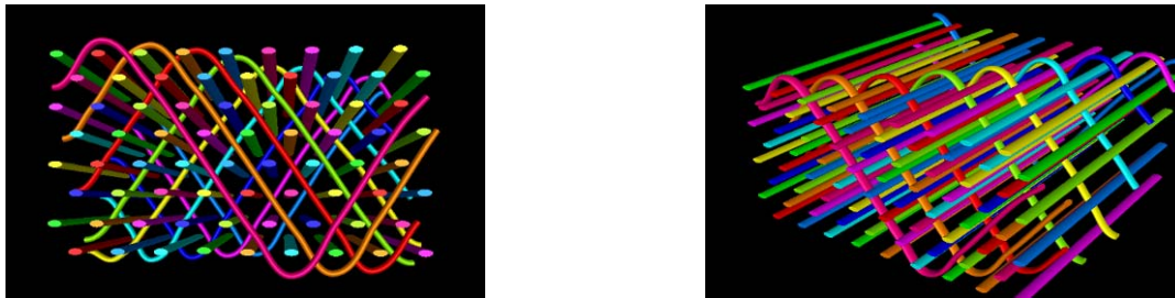
Fig. 3 Left: cross-section of the through-the-thickness angle interlock. Right: 3D modeling view with 9 warp yarns and 8 layers of weft yarns.
