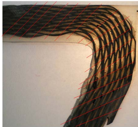
Fig. 13 Intermediate phase of angle interlock deformation.
