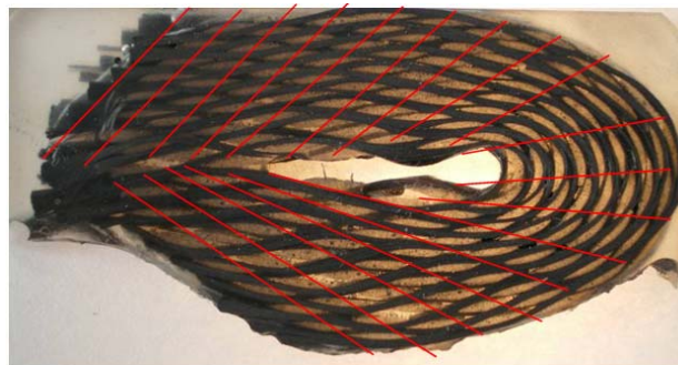
Fig. 14 Final phase of the total deformation of angle interlock.
